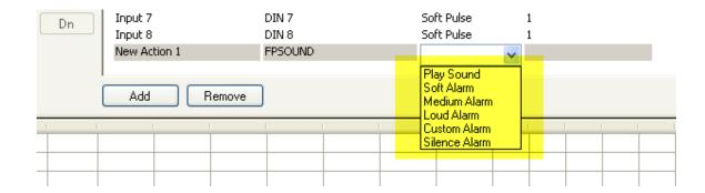
**Play Sound** – this will play a 'raw' sound file that is stored in the JNIOR Control Panel. The Control Panel includes one sample called Sound3.raw. INTEG will be providing more updates and information related to this feature. With the current software release, you can put 3 in the data column and this Action will then play the Sound3.raw file when the macro is executed. This feature is being developed should the user have their own sounds they would like to use.
