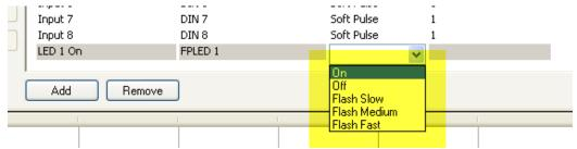
With the Flash function (Slow, Medium, Fast) you can add a value in the last column (the data column) that will indicate the number of times the LED should flash. If you leave the data column blank, then the LED will flash until the Off action is received. If you enter a number, the LED will flash that many times.
